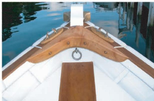
Clinker construction with steam bent ribs and grown knees.
